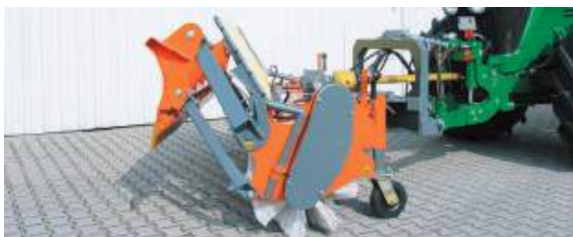
bema Snow-Combi, traktormontering (trepunktsbukk)
