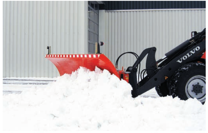
bema Snow plough series 1100, wheel loader attachment (quick-change mounting)
