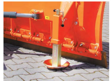
Version 2: Spring flaps & skid plates
