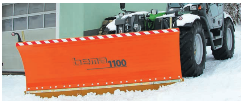
bema Snow plough series 1100, telehandler attachment (quick change adapter)
