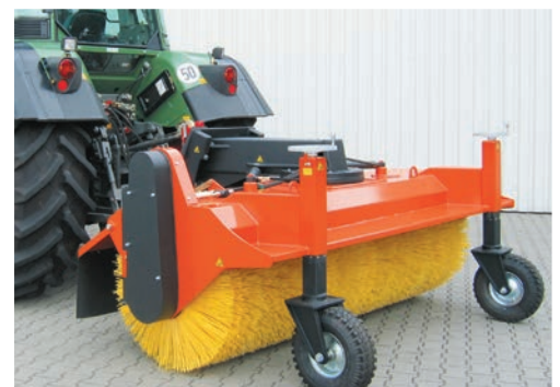
bema Jumbo on a tractor rear (three point linkage / rear)
