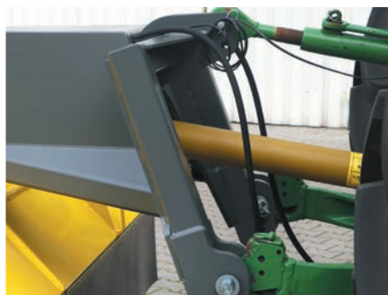
Pendulum compensation (three point linkage/rear)
