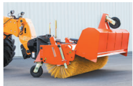
bema 30 Dual PowerMaster attached on wheel loader, collection container Dual opened
