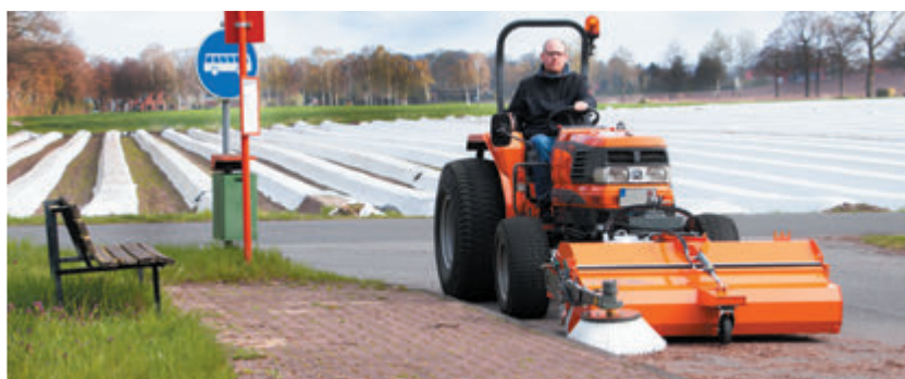
bema Kommunal 580 Dual with rotary side brush - ideal for kerbs, gutters and on buildings
