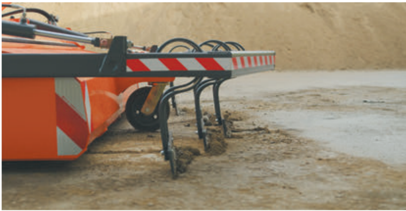
Scraper bar is divided into several Hardox segments
