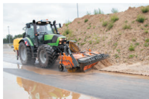
bema 75 Dual PowerMaster with scraper unit instead of collection container (see page 58/59)
