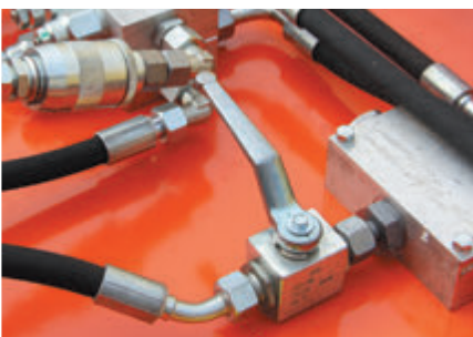
Adjustable restrictor & quantity divider (even lifting of the snow plough)
