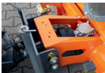
bema Suction sweeper drive via front power take-off (optionally available)
