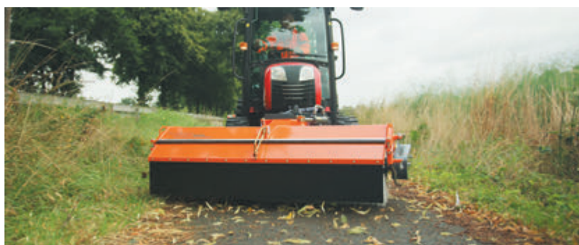
bema Kommunal 450 Dual with protection cover (without collection container/free sweeping)
