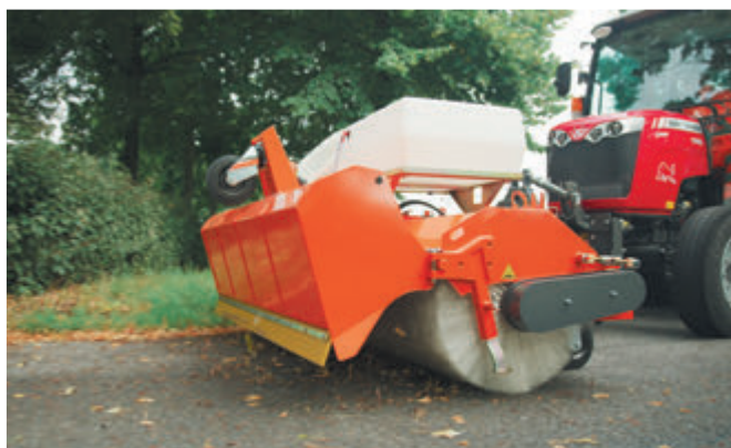
Collection container in Dual system - very quick change between free sweeping and collecting dirt
