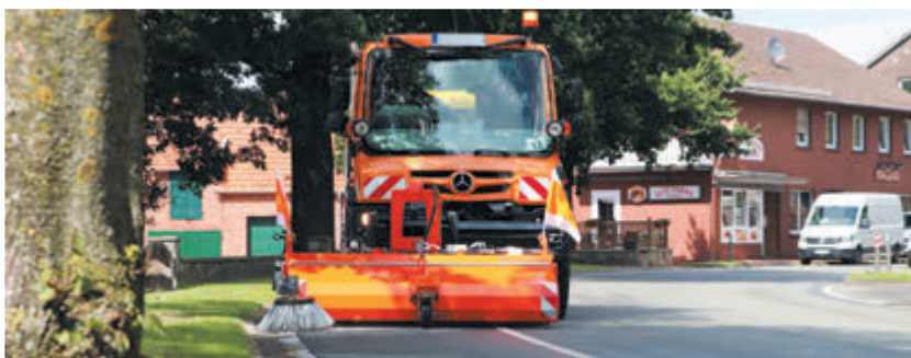
bema 30 Dual PowerMaster attached on Unimog with rotary side brush and hydraulic lateral movement (500 mm to the left/right)
