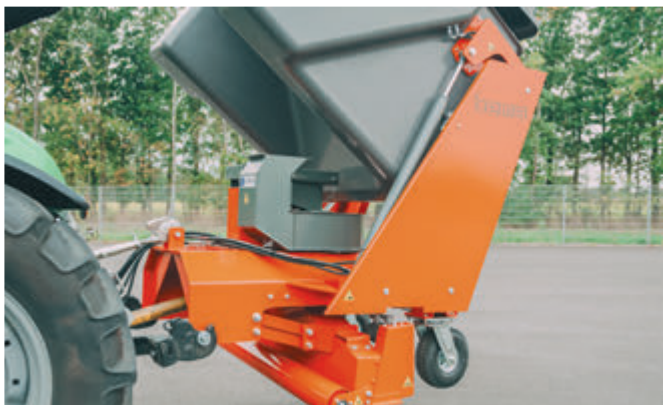
Complete rear unit consisting of bema Suction sweeper, chaff blower and bema Tipping container
