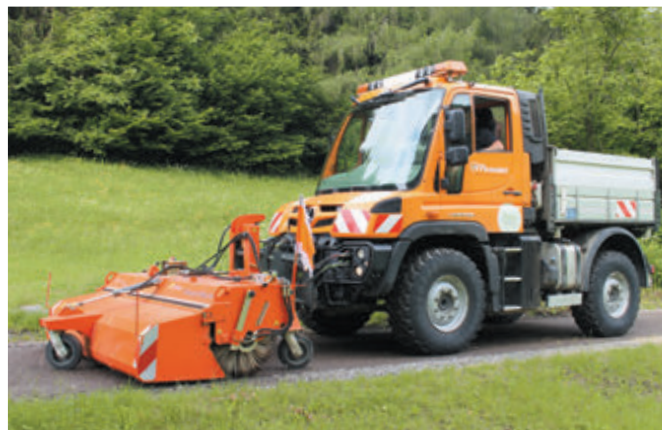
bema 35 Dual PowerMaster in municipal use, Unimog attachment
