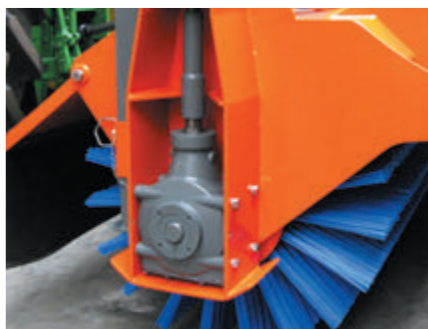
Gearbox (on the side)
