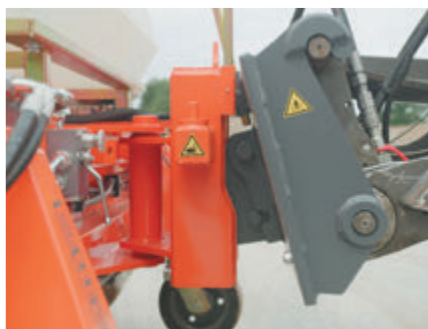
3D roller level compensation and optional swivel joint
