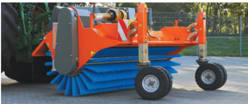
bema Jumbo Airport at tractor rear, special construction with hydraulic support wheel adjustment
