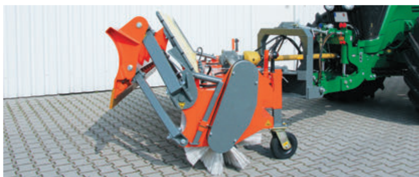
bema Snow-Combi, tractor attachment (three point linkage)
