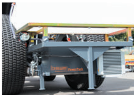
bema PowerPack with oil cooler and water tank in the rear
