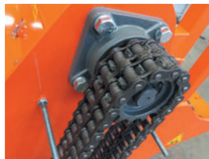
Mechanical drive via duplex chain
