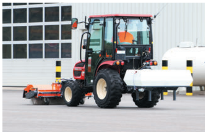
bema Kommunal 450 Dual with water tank in the rear
