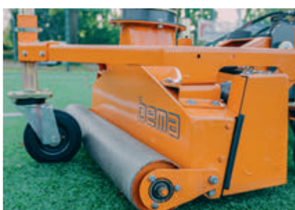
Trouble-free feed by pendulum mounted downholder roller (feed roller)
