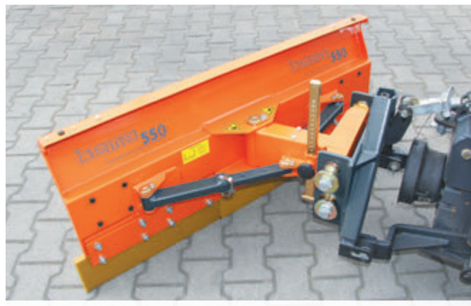
bema Snow plough series 550, mechanical angle adjustment
