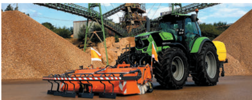
bema Scraper unit with collection container in combination with bema High-pressure water unit and water tank (2000 litres in the rear)
