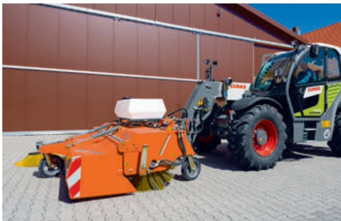
bema 75 Dual PowerMaster on telehandler, quick change adaptor
