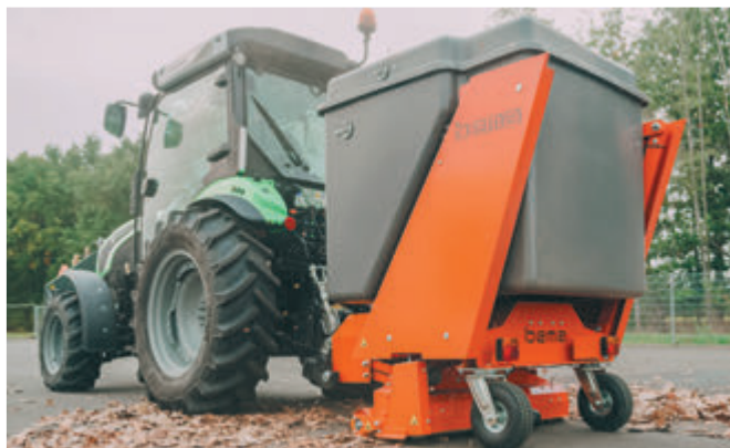
The complete rear unit is quickly ready-mounted with three-point linkage Cat. I/II
