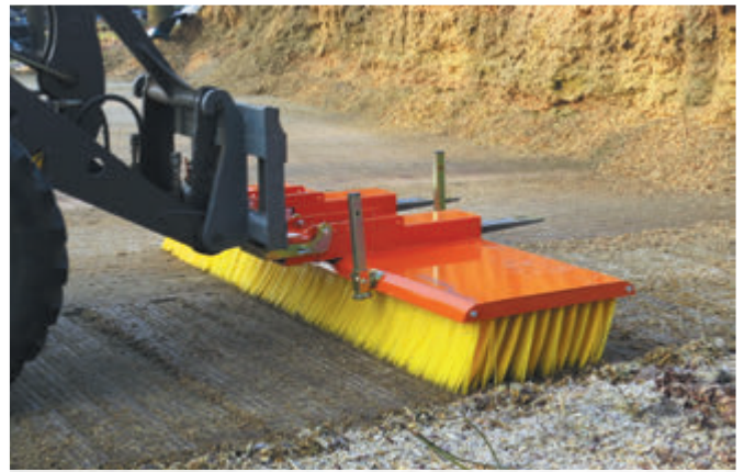
Pushing silage with the bema 11 Multi-Clean
