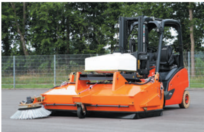
bema 40 Industry with rotary side brush and water spray unit
