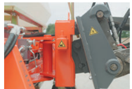
3D roller level compensation and optional swivel joint
