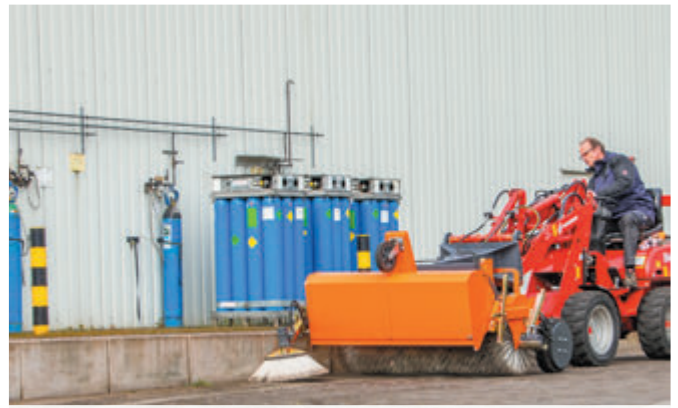
Collection container featuring the proven Dual system e.g. free sweeping with an opened collection container
