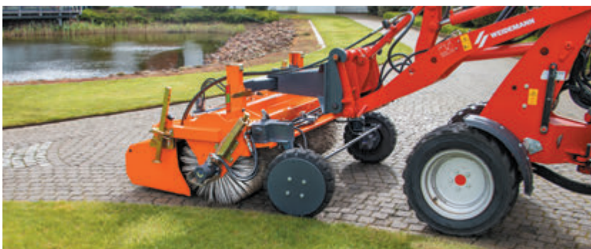
Featuring two steerable wheel-drives, the sweeper is independent from the carrier vehicle.
