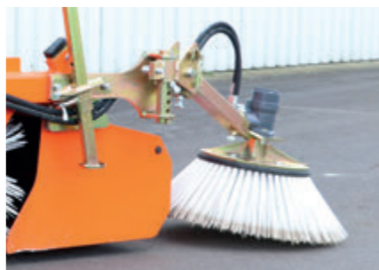
Rotary side brush, alternatively on the right or the left side
